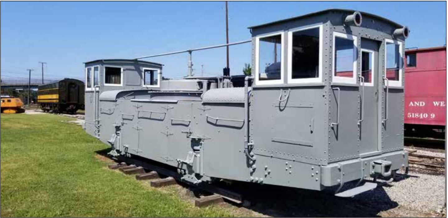
Transportation. The last of the metalwork, bodywork, and rivet replacement have been completed. The marker lights and cab lights have also been rewired so that they can work off of an extension cord. Over the Labor Day weekend, we were blessed with cooler, drier weather and were
