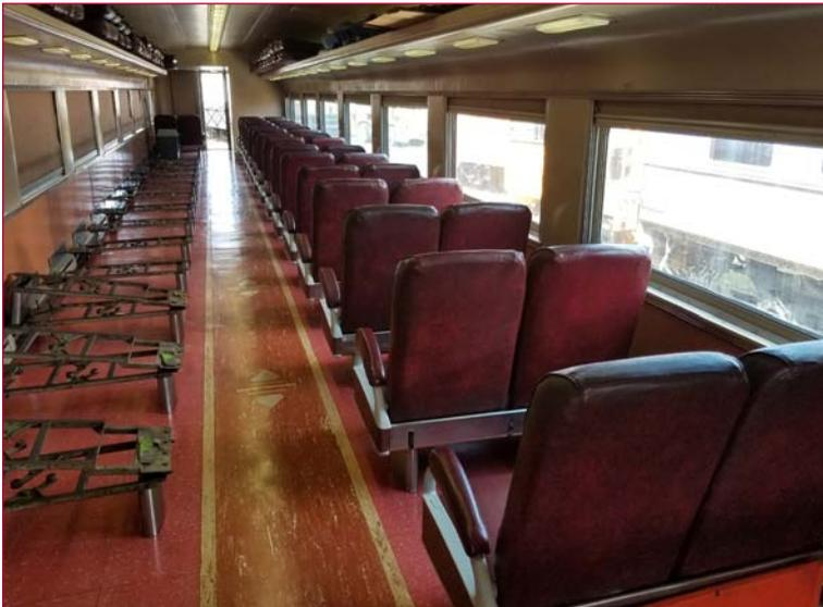
assembled to install the stainless steel kick plates on the back of the seat. This process is about 1/3 done at this point, and we hope to finish up in a couple of weeks. We've also added a few details, like the nickel-plated trim around the sink in the restroom. While not laid out as it was built, the restroom definitely feels much more original.
